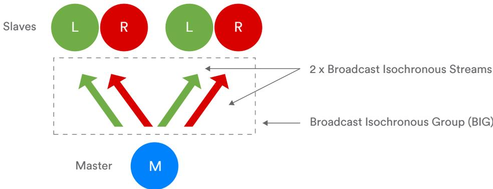
Figure 11 - Broadcast isochronous stream and group
