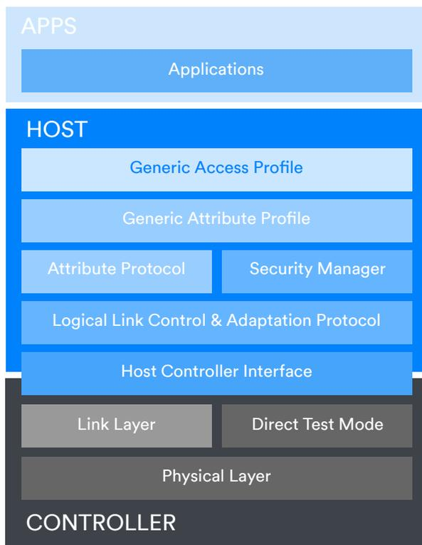
Figure 1 - Bluetooth LE with GATT, GAP, and ATT
