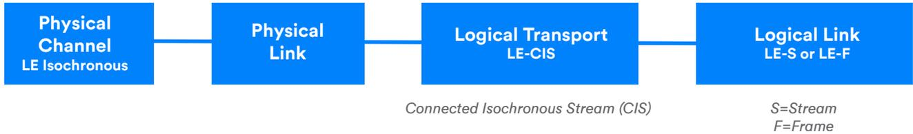
Figure 7 - Connection-oriented isochronous channel data transport
