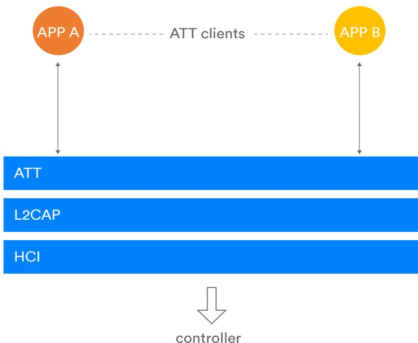
Figure 3 - Two applications using the same stack
