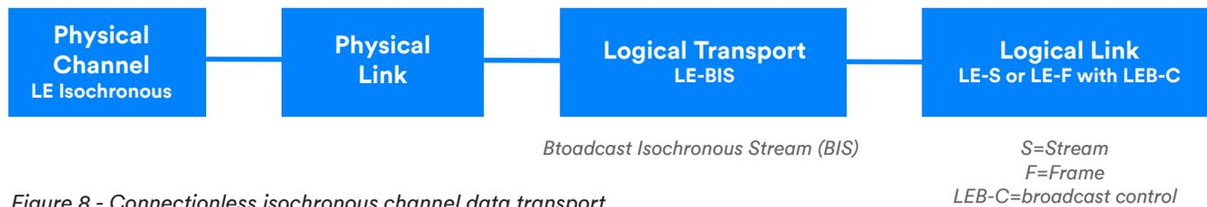
Figure 8 - Connectionless isochronous channel data transport
