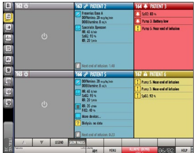
A sample screenshot of Digistat® Smart Central, showing 6 beds with patient vital signs from monitor, ventilator and infusion pumps including some alarms and warnings.
