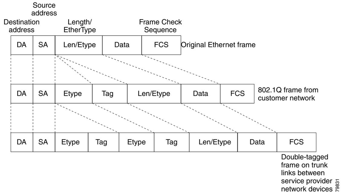
When a tunnel port receives tagged customer traffic from an 802.1Q trunk port, it does not strip the received 802.1Q tag from the frame header; instead, the tunnel port leaves the 802.1Q tag intact, adds a 2-byte Ethertype field (0x8100) followed by a 2-byte field containing the priority (CoS) and the VLAN. The received customer traffic is then put into the VLAN to which the tunnel port is assigned. This Ethertype 0x8100 traffic, with the received 802.1Q tag intact, is called tunnel traffic.
